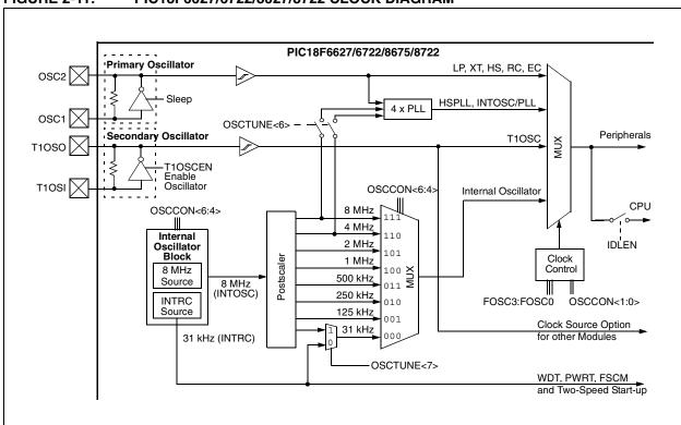
FIGURE 2-11: PIC18F6627/6722/8627/8722 CLOCK DIAGRAM
