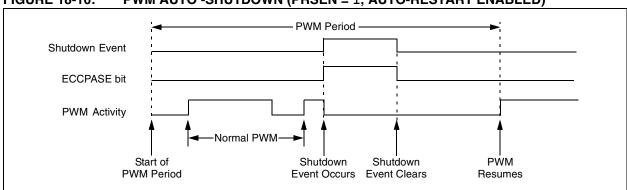
FIGURE 18-10: PWM AUTO -SHUTDOWN (PRSEN = 1, AUTO-RESTART ENABLED)
