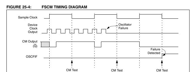
**Note:** The device clock is normally at a much higher frequency than the sample clock. The relative frequencies in this example have been chosen for clarity.
