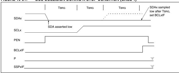
FIGURE 19-32: BUS COLLISION DURING A STOP CONDITION (CASE 2)
