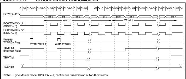
FIGURE 20-12: SYNCHRONOUS TRANSMISSION (THROUGH TXEN)
