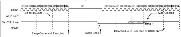
Note 1: If the wake-up event requires long oscillator warm-up time, the auto-clear of the WUE bit can occur before the oscillator is ready. This sequence should not depend on the presence of Q clocks.
