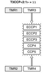
Timer3 is used for all Capture and Compare operations for all CCP modules. Timer4 is used for PWM operations for all CCP modules. Modules may share either timer resource as a common time base.
