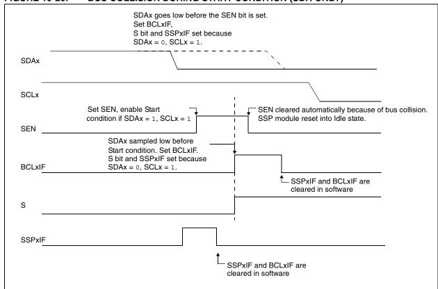
FIGURE 19-27: BUS COLLISION DURING START CONDITION (SCL = 0)
