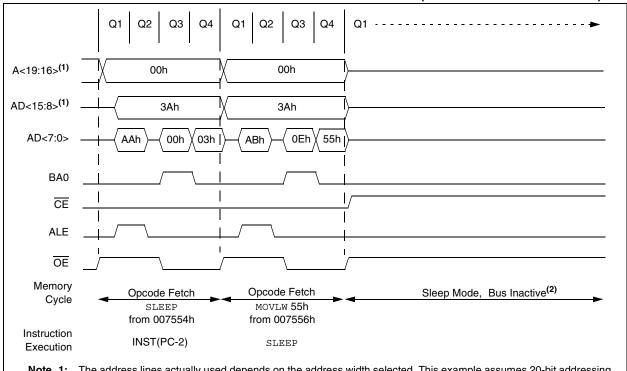
Note 1: The address lines actually used depends on the address width selected. This example assumes 20-bit addressing.
