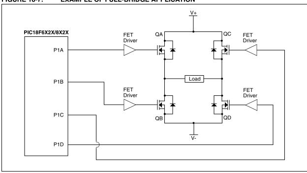
FIGURE 18-7: EXAMPLE OF FULL-BRIDGE APPLICATION
