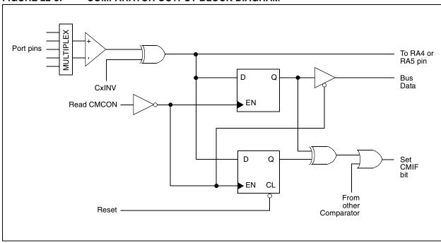
FIGURE 22-3: COMPARATOR OUTPUT BLOCK DIAGRAM
