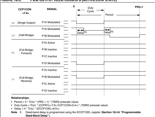
FIGURE 18-3: PWM OUTPUT RELATIONSHIPS (ACTIVE-LOW STATE)
