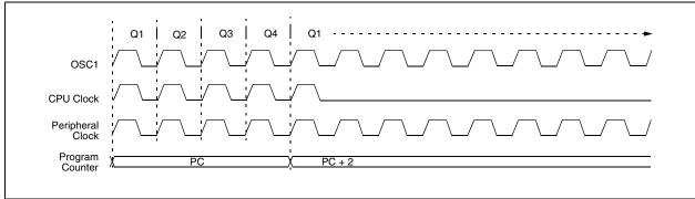
FIGURE 3-8: TRANSITION TIMING FOR WAKE FROM IDLE TO RUN MODE
