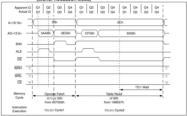
FIGURE 7-5: EXTERNAL MEMORY BUS TIMING FOR TBLRD (EXTENDED MICROCONTROLLER MODE)
